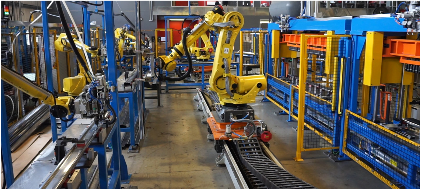
A transfer station between the halves of the work cell allows all five robots to operate in unison to accomplish multiple tasks with the lowest possible cycle times.
